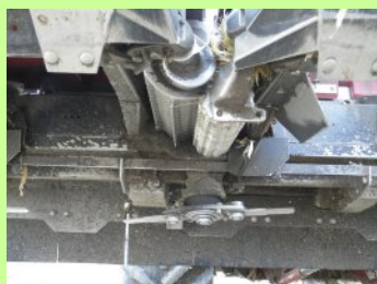
Geringhoff: Horizon Star: shredding disks with 2-blade choppers whose axle is behind the rollers.
