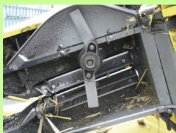
New Holland: 2-blade chopper with its axle at the side of the rollers.
