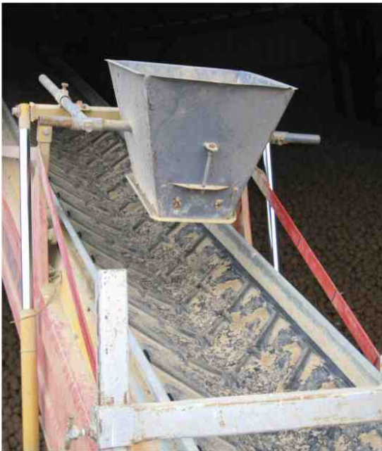
Tuber dusting with CIPC on the conveyor belt as the heap is being formed, achieves a simple and effective sprout control treatment if required
