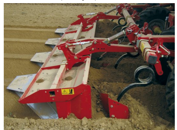
Creating a ridge at the time of planting using a suitable bed-former fixed behind the planter requires a sufficient volume of crumbly soil.
