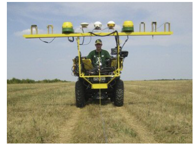
In order to assess each of the differential corrections available on the French market, they were tested simultaneously at the Boigneville research station (South of Paris).
