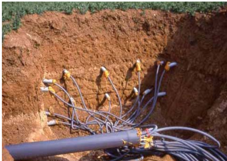
The bundle of seven porous cups laid out at the beginning of the trial (1991) and the network of capillary tubes to collect the soil solution
