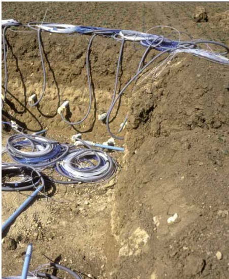
Porous cups are laid out to collect the soil solution.
