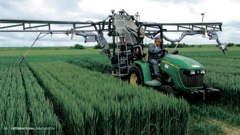
four identical spectrometers are fitted onto a boom and measure hyperspectral reflectance. While one spectrometer measures irradiance, another is angled toward the nadir at the zenith position and two sit on either sides of the sampling area. In addition, there are also cameras for measuring the green fraction of leaves. All of Arche's onboard devices are automatically triggered using real-time, centimetre accurate, geolocation technology.
