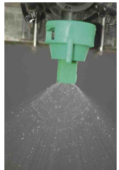
It is possible to use nozzles that do not tend to cause much spray drift (air induction), without affecting the efficacy of the treatments. It is also possible to use them with lower volumes/ha.
