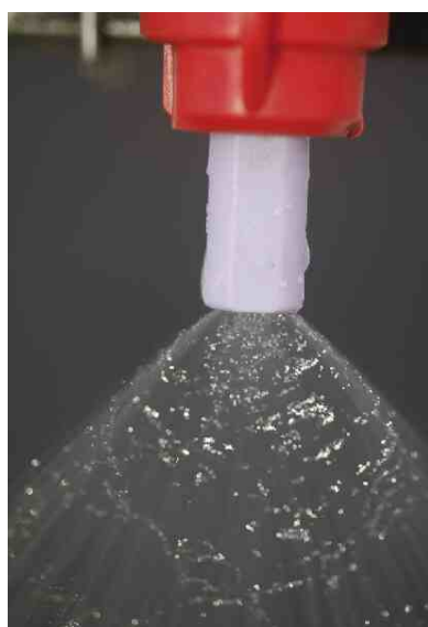
Air induction" technology introduces air bubbles into the droplets, which greatly increases their diameter.
