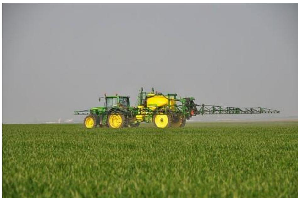
GPS can optimise the whole field when boom section shut-off is combined with homing guidance.
