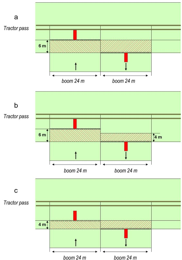
If the driver shuts off the whole boom when the front wheels of the tractor cross the first wheeling in the headland, there will be a double treatment over a length of about 6 m.
