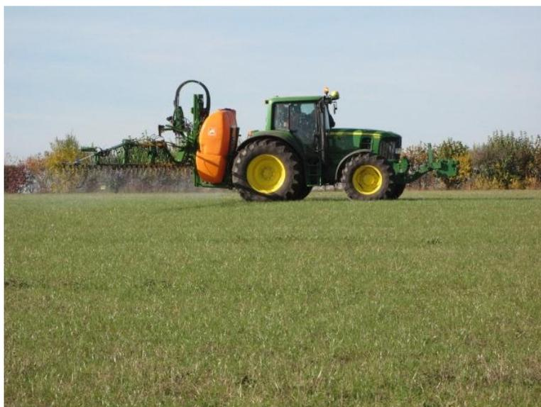
*The greater the number of spray-boom sections, the smaller the area of overlap.*
