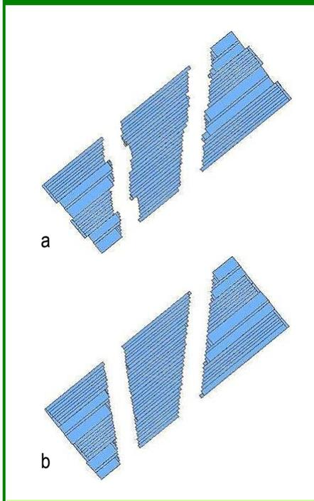
The boundary between the zones already sprayed is more even when the sections are shut off by the GPS. The overlaps are visually less obvious.
