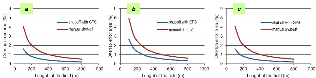
The gain in area due to the use of GPS is greater on the rectangular plot, being 2.7 % for a field 100 m long.
