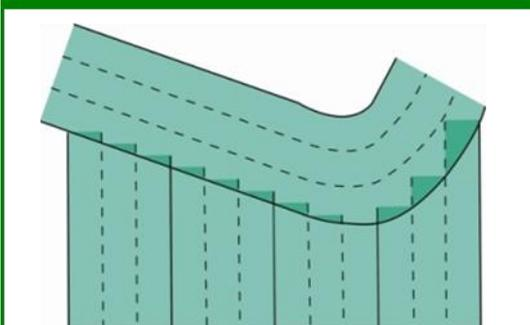
The objective of the system is to optimise the overlaps (and the unsprayed areas) with the zones already treated.
