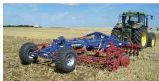
The design of modern disc harrows with a roller ensures perfect depth control.
