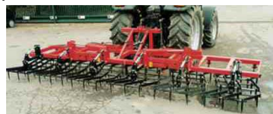
A heavy harrow is a fairly simple tool which, through its compartmented design, is able to adjust to the topography of the land.
